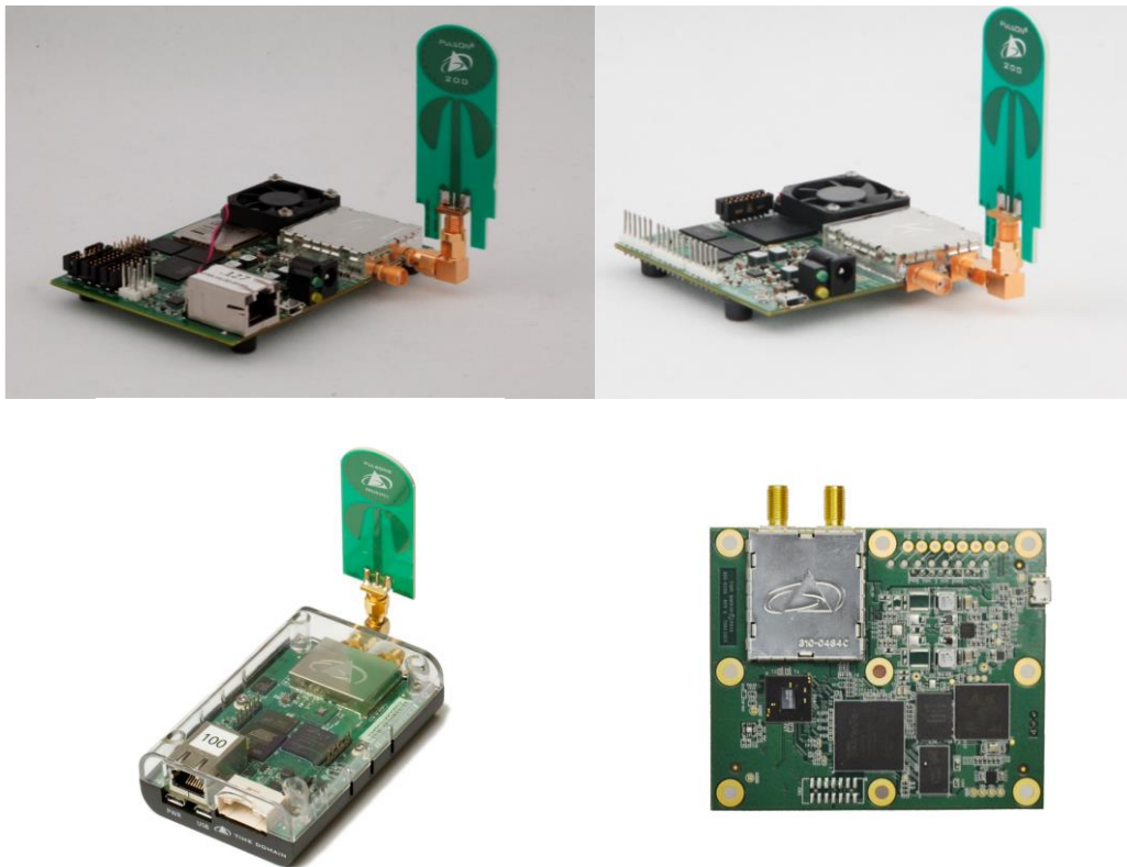
Fig. 1: Clockwise from upper left P400, P410, P412, and P440 (shown with attached BroadSpec Antenna)
