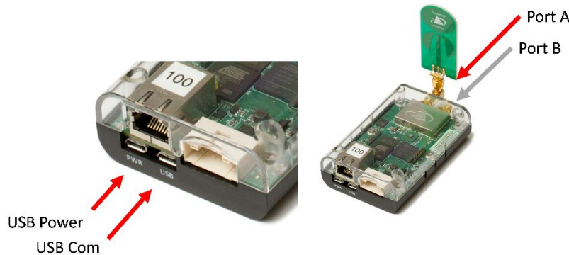
Fig. 4: Side view of the P440 module showing the various connections
