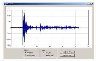
Fig. 3. GUI screen capture illustrating typical channel impulse response/bistatic radar scan.
