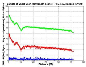
Fig. 6. Sample code allows plotting of range vs Signal strength, SNR and noise.
