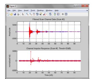
Fig. 9. Converting captured waveforms into channel impulse response
