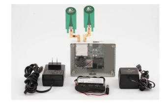
Fig. 1. P400 shown with supply, battery and chargers.
