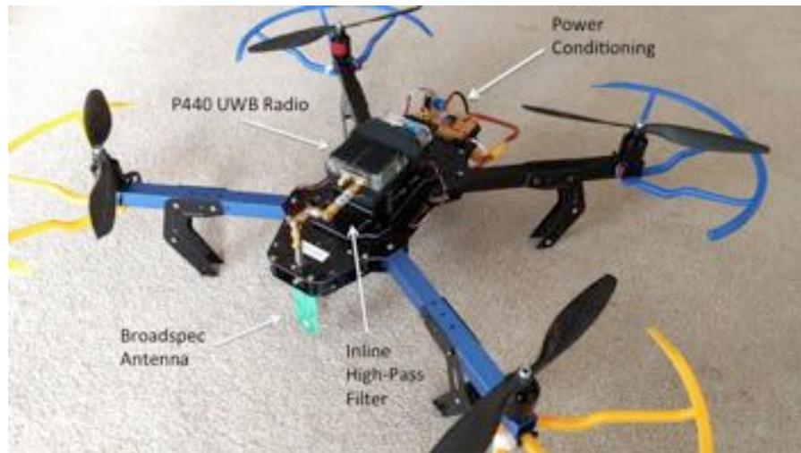
**Figure 6. Quadrotor platform with P440 UWB radio**
