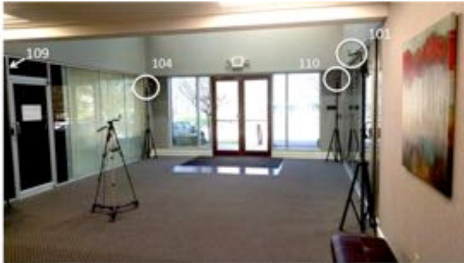
**Figure 5. Indoor test area with anchor setup**
