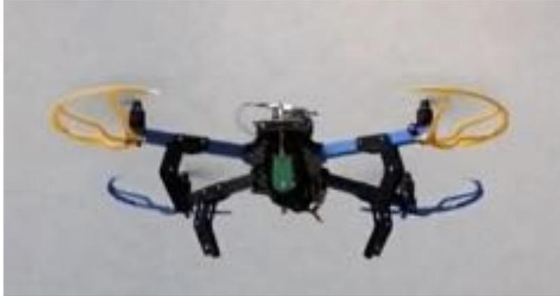
**Figure 1. UWB radio mounted on quadrotor in flight.**
