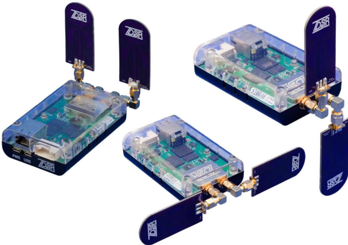
Fig. 1: P452 MRM with attached BroadSpecs showing 3 Antenna Configurations
