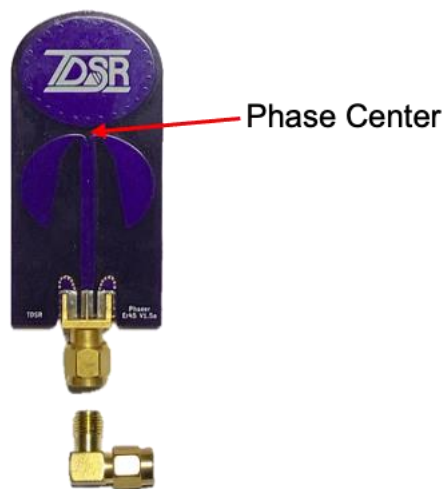
Fig. 7-1: BroadSpec antenna with phase center indicated
