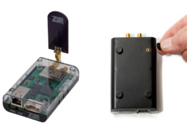
Fig. 4-12: P452 in standard enclosure (left) and view of enclosure bottom showing feet and mounting holes for 4-40 screw
